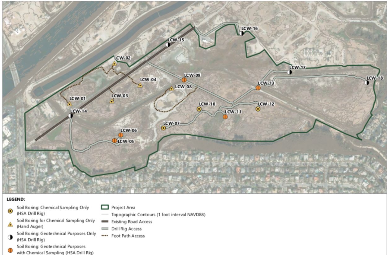
Figure 8 map of proposed Drill Rig Access and Foot Path Access (which do not currently exist).
