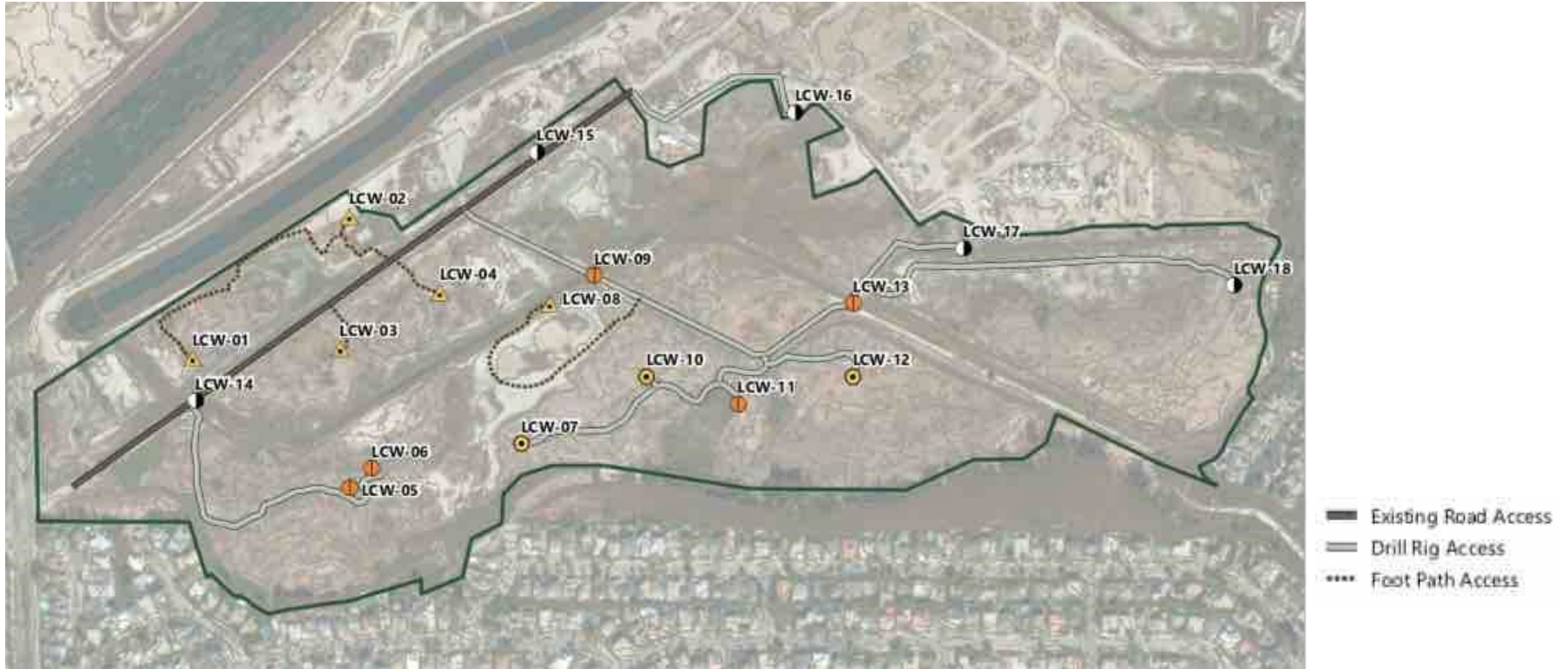
Figure 8 Map of includes Drill Rig Access to boreholes 5,6,7,10,11,12 and foot path access routes to 1,2,3,4,8. These routes do not now exist and would be made by removing existing vegetation.
