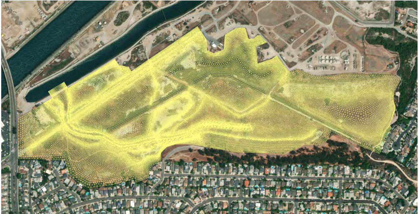
Figure 5: Model Mesh for the Southern LCW Restoration, Phase 2
